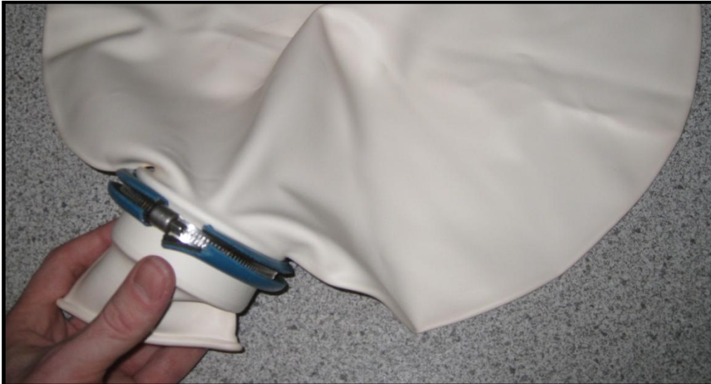
Figure 17 - Attaching the clamping band on the balloon mount.
