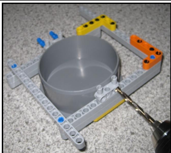
Figure 5 - The drill guiding construction in action.
