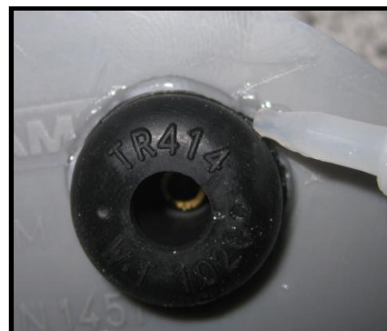
Figure 12 - Applying the glue after pulling the valve through the hole.
