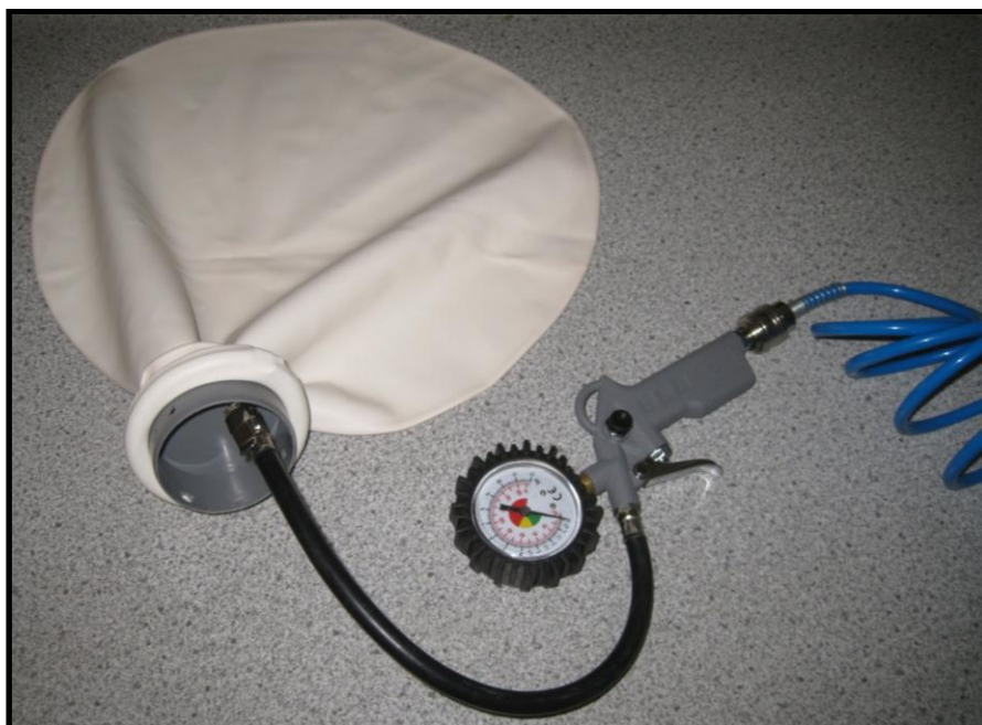
Figure 23 – Using the tyre inflating gun allows us to fill the balloon through the valve we fitted onto the balloon mount.
