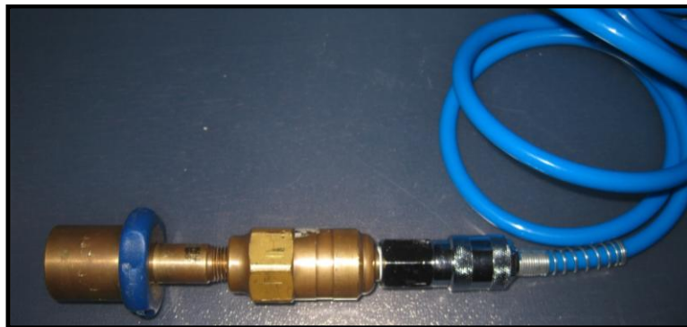
Figure 22 - Attaching a standard pneumatic hose to the quick coupling.
