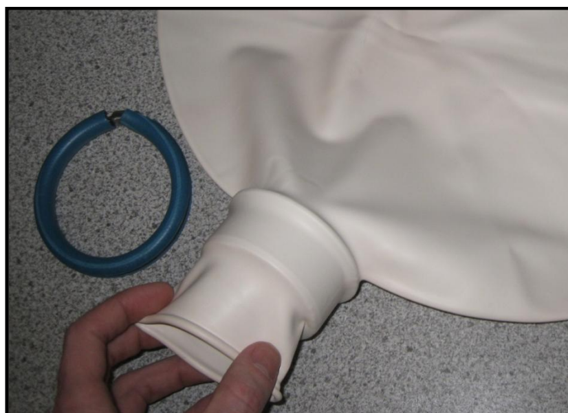
Figure 16 - Mounting the balloon on the balloon mount.
