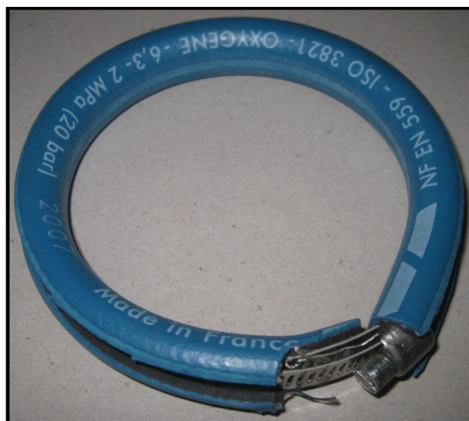
Figure 14 - Clamping band with protective rubber hose.
