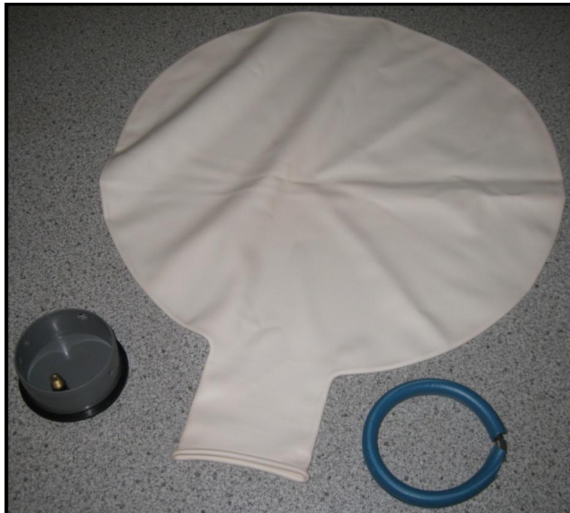
Figure 15 - Balloon with the balloon mount and the clamping band.
