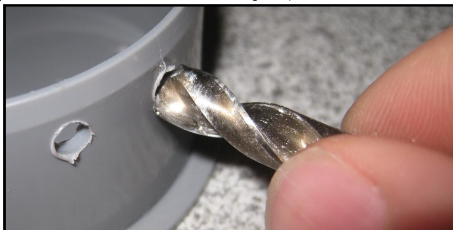
Figure 7 - Removal of sharp edges around the holes.
