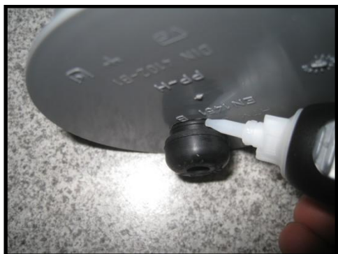
Figure 10 - Applying the glue before pulling the valve through the hole.
