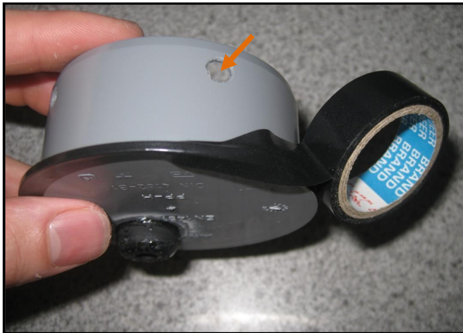
Figure 13 - Applying electrical tape to the plug.
