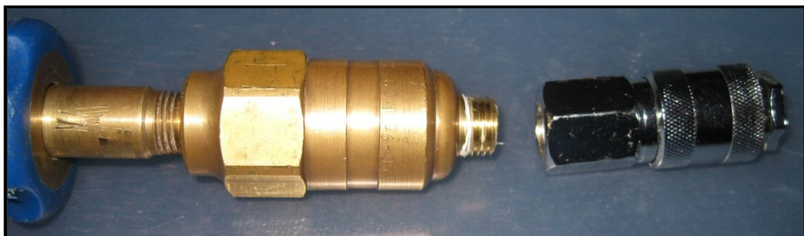
Figure 20 - The pressure reduction valve and the pneumatic quick coupling.
