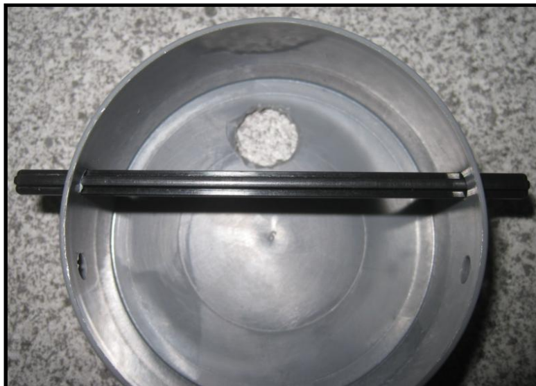
Figure 9 - Placement of the valve.
